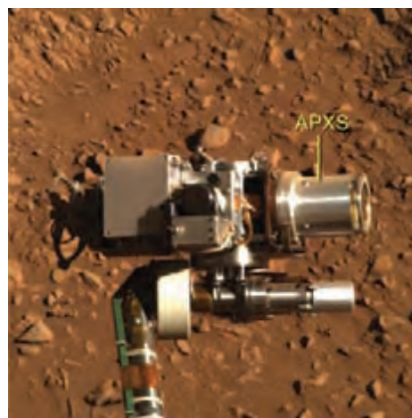
Figure 4.1. MER Alpha Particle X-ray Spectrometer (APXS). Sensor head (label) is mounted on the turret (lower part), which is attached to the instrument deployment device (arm on the bottom). (Picture taken at Gusev crater on sol 287 by Pancam [NASA/JPL, Cornell].) (For a color version of this figure, please refer to the color plate section or to the e-Book version of this chapter.)
