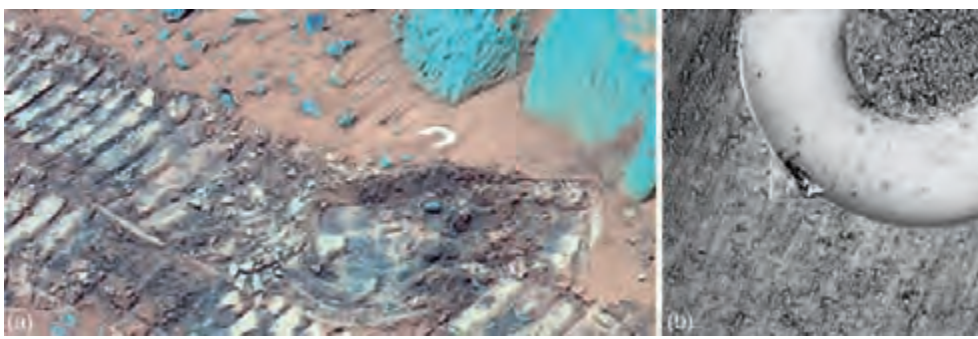
Figure 20.7. (a) Spirit Pancam false-color view of tracks and Mössbauer imprint into dusty aeolian drift material, obtained near the summit of Husband Hill on Sol 589. Pancam filters are L2 (753 nm), L5 (535 nm), and L7 (432 nm) stretched into red, green, and blue, respectively. The Mössbauer imprint is the bright, partial ring feature at central upper-right in this view. (b) Spirit MI image of the same Mössbauer contact plate imprint, obtained on Sol 588 in full shadow. The MI was rotated at the time of imaging relative to the orientation of (a). MI view is ~31 mm across.
