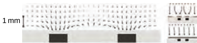
Figure 16.15. The principle of the Sweep Magnet experiment on MER. (left) A vector field illustrating the magnetic field gradient (effectively the magnetic force) as a function of radial distance from the center of the magnet. The gray box illustrates the aluminum structure of the magnet and the dark gray boxes embedded in the structure illustrate the samarium-cobalt ( \text{Sm}_2\text{Co}_{17} ) magnetic material. Note that the force is slightly repulsive in the center of the magnet. (top right) A figure illustrating how the paths of magnetic dust grains settling out of the atmosphere are deflected as a result of interaction with the magnet and (bottom right) how nonmagnetic dust grains settle on the magnet. (For a color version of this figure, please refer to the color plate section or to the e-Book version of this chapter.)
