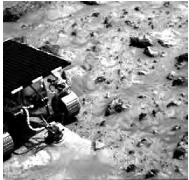
Figure 20.4. IMP image of Sojourner rover performing APXS measurement of “Scooby Doo,” a hard, indurated, soil-like deposit whose elemental composition is similar to other soils but which was not noticeably scratched or marked during “road warrior” rock wheel scratch tests.
