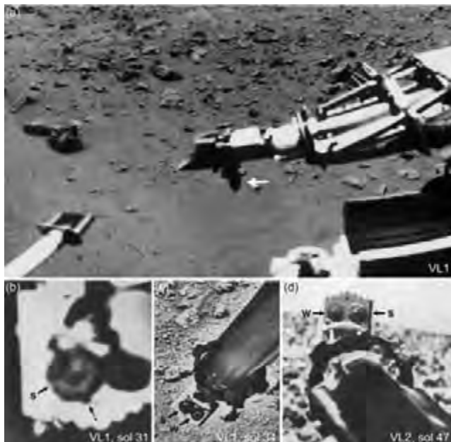
Figure 16.4. Magnets (arrows) on the backhoe of the Viking Lander soil sampler. (a) Location of the backhoe on the Viking Lander 1 sampling arm. (b–d) View of backhoe and backhoe magnets at different times during the mission. Weak (w) and strong (s) magnets hold similar amounts of material. Viking Lander 1 images (b, c) were acquired after six insertions into the soil. Note the protrusion (dotted arrow) near the periphery of the particle accumulation likely caused by an \sim 2 mm large magnetic particle. Viking Lander 2 image (d) was acquired after eleven insertions into the soil. The height of the particle accumulations on both magnets is estimated to be 2–4 mm.
