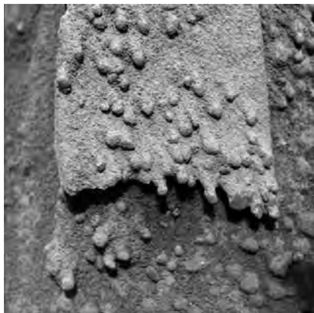
Figure 20.14. Opportunity MI image 1M173457602IFF55W4P29-36M2F1 obtained where Opportunity became severely bogged (embedded) while climbing an unusually large ripple, informally dubbed “Purgatory.” This view, about 31 mm across, shows part of a tablet of soil compacted and remolded by the wheel cleats, then deposited alongside a track. Hematitic spherules (interpreted as concretions) 1–2 mm in diameter have been incorporated into this wheel-made, molded clod. They were mixed with and embedded within a finer, poorly sorted soil matrix that acquired slightly cohesive properties when compacted by the wheel. After creation, the tablet was subjected to aeolian erosion of the matrix, exposing the 1–2 mm concretions, particularly along the tablet’s lower edge (note pedestals). During Opportunity ’s ~40 sol stay in this area, wind events were seen to affect only areas disturbed by the rover, such as this example viewed on Sol 510.
