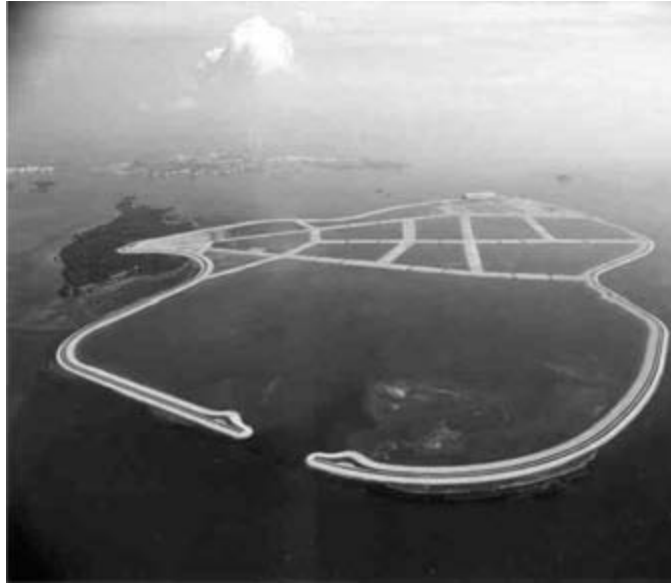
Fig. 3.2 Pulau Semakau – Singapore's landfill island. Land scarcity and increasing demand for waste disposal sites led to the construction of the new $S610 million landfill at Pulau Semakau. As this aerial view shows, the majority of the landfill is 're-claimed' land. Photograph courtesy of the Ministry of the Environment, Singapore.
