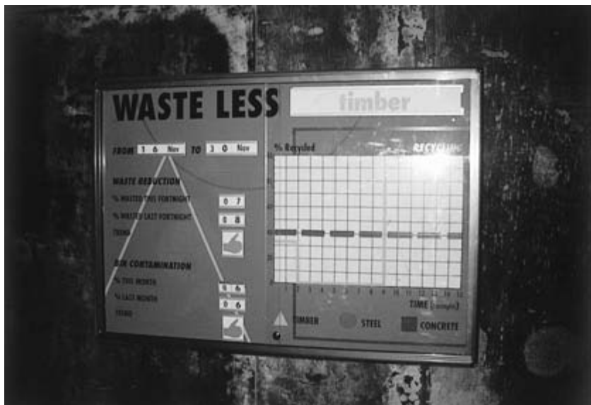
Fig. 7.2 'Waste less' sign. Feedback for workers on their performance helps achieve the best results on-site. These signs were erected during construction of the Docklands Stadium project in Melbourne Australia. Every two weeks the quantity of material sent to land fill was compared with the quantity sent off-site for recycling. The two figures were compared in relation to the quantity of material, in this case timber, being used on-site during that period. Increased recycling rates got a thumbs up, decrease got a thumbs down. Supervisors were then asked to set targets for recycling for the coming two-week period. The target is shown as a dashed line. Actual performance in relation to the target was then plotted to provide feedback on recycling performance. Reference: Lingard, H., Smithers, G. & Graham, P. (2001) Improving solid waste reduction and recycling performance using goal setting and feedback. Construction Management and Economics 19 809–817.
