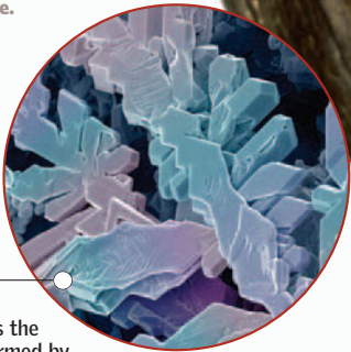
Microphotograph of silver crystal dendrites
