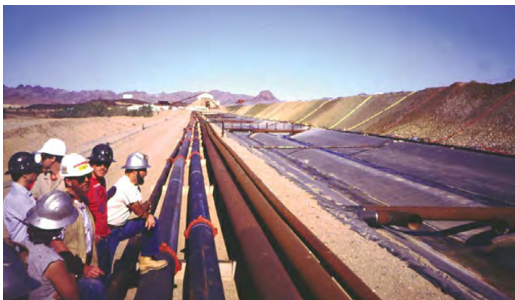
Figure 5 Heaps of low-grade epithermal gold ore are piled on black plastic mats and sprinkled with sodium cyanide solution at the open-pit Mesquite Mine, Imperial County, California, USA. One set of steel pipes delivers fresh solution to the sprinkler systems atop the heaps, while the other set carries away 'pregnant' gold-laden cyanide liquor that drains from the heaps and accumulates in the trenches.
