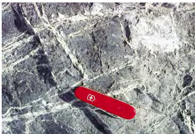
Figure 12 A network of cross-fibre chrysotile asbestos veins in serpentine, Havelock mine, Swaziland. This length of fibre and intensity of mineralization constitutes superior grade ore. Photo: GR Davis.
