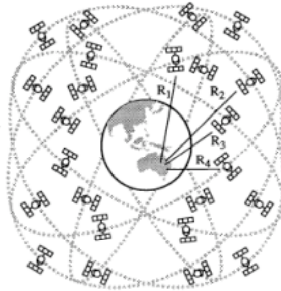
Figure 1.7: The GPS Constellation "Birdcage".
