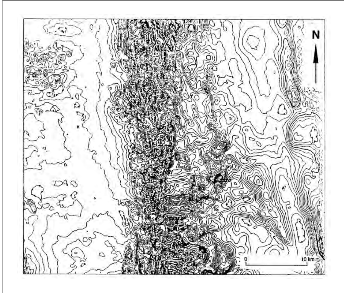
Figure 6.2 Contour map of magnetic anomalies for a survey flown at 100 m ground clearance, east-west lines at 400 m spacing and a contour interval of 2 nT. Relatively magnetic metasediments occupy the centre of the map, with a granite body to the east and sediments to the west (Courtesy of the Australian Geological Survey Organisation)
