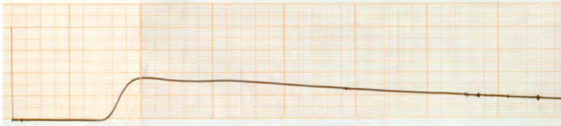
Figure 6: Graph showing the typical pressure pulse for one of the internal monitoring wells (FT-2, FT-4, Ft-6 and 0.10 psig full scale, 1mm/sec)).
