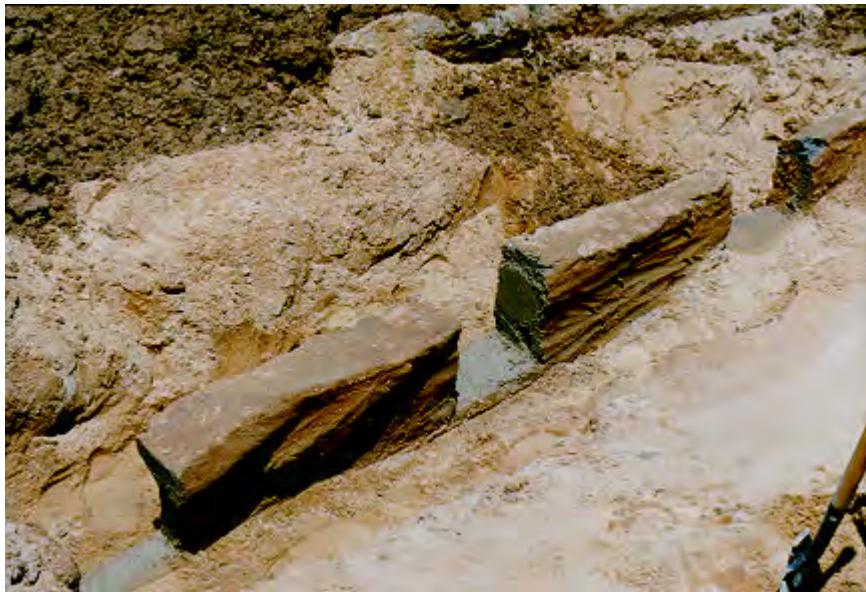
Figure 3: A picture showing an excavated thin diaphragm panel emplaced using high pressure jetting.
