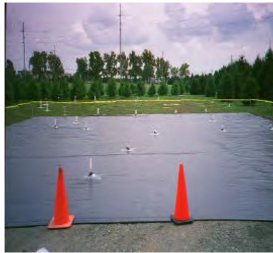
Figure 2: A picture of the geomembrane cover and piezometers.
