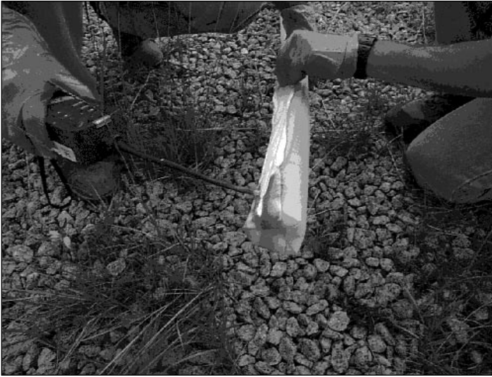
Figure 3-34. Picture of FLUTE™ membrane recovered from a CPT borehole. Dark marks indicate DNAPL at that depth.
