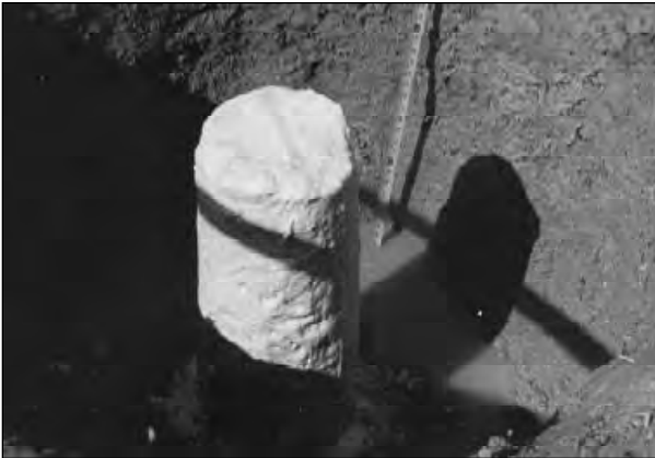
Figure 5. Intact core collected from the shallow vadose zone by perimeter carving and wax encapsulation.
