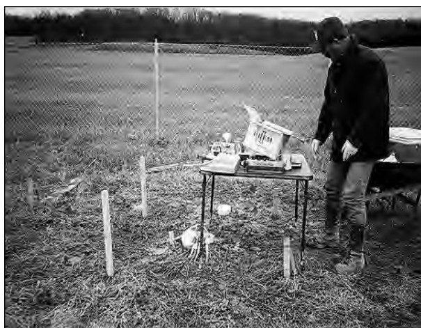
Figure 3. Monitoring vadose zone sensors and lysimeters in the zero valent iron cell.
