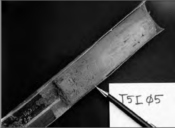
Figure 4. Intact soil core collected from the permanganate cell illustrating presence of oxidant (redox along the entire core length was elevated above 800 mv).
