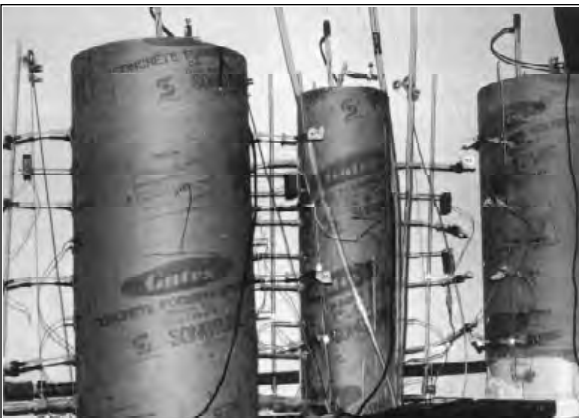
Figure 6. Intact cores established in the laboratory at CSM on porous tension plates and instrumented with moisture and redox sensors.
