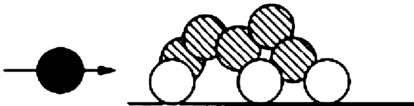
Fig. 11. A schematic diagram illustrating the mechanism for large-avalanche formation. When \Delta is large, there is a great deal of undissipated volume in the cluster, resulting in the upper ( shaded ) grains being unstable to small perturbations. When \alpha is large, the black grain hitting the cluster has large inertia so that a large avalanche results when it dislodges the shaded grains
