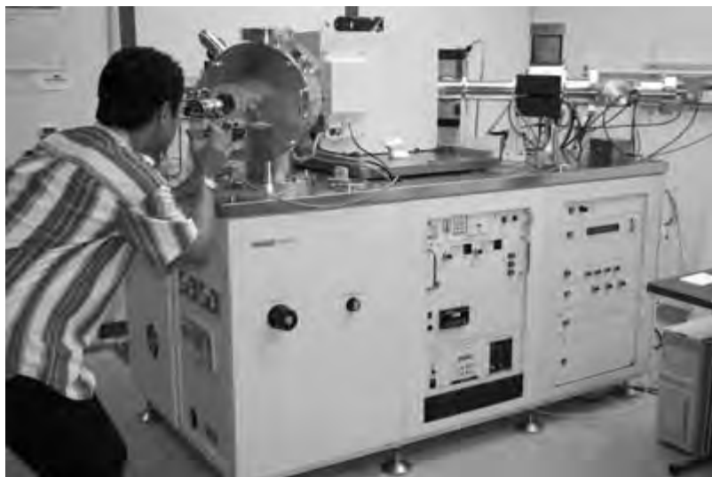
Figure 26. A mass spectrometer at the Scripps Institution of Oceanography of the University of California at San Diego. Samples are placed in the chamber into which geologist Pat Castillo is peering. Ions produced by heating are sent along a stainless steel tube through the magnet (large gray block, top center), where they are deflected along a curved path into collectors at the top right of the picture. Photo courtesy of Pat Castillo.
