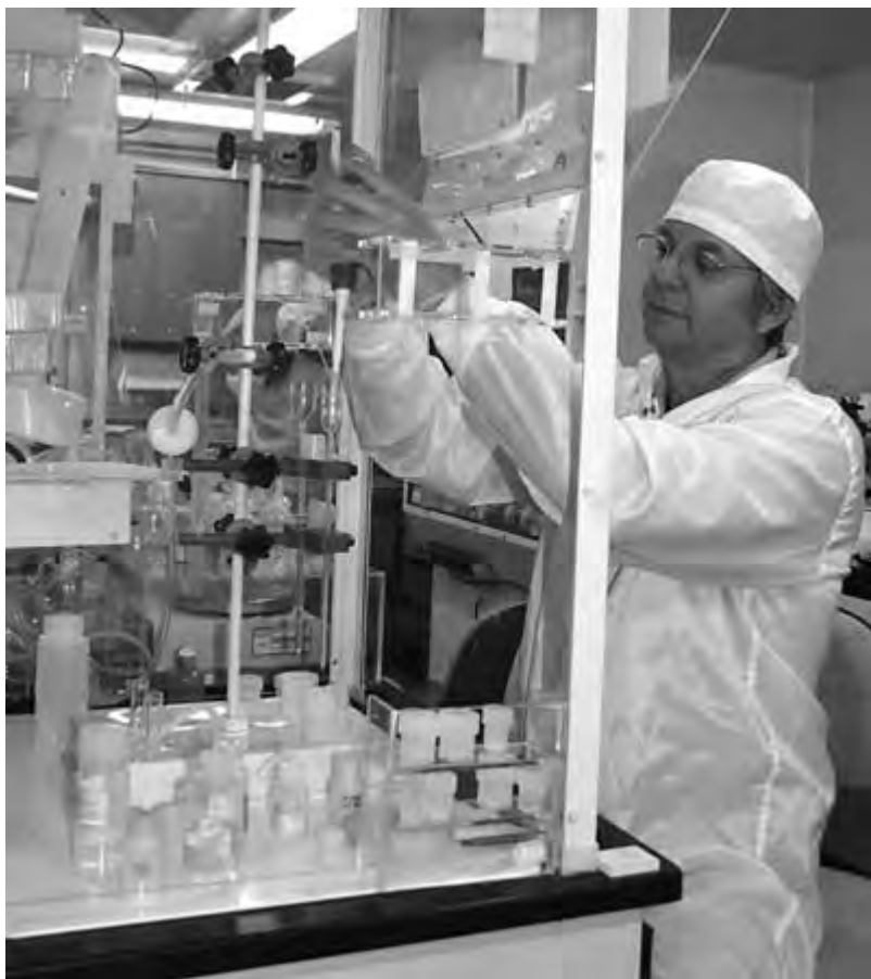
Figure 18. Researcher Chris MacIsaac, garbed in lint-free lab clothing and working in an enclosure bathed in filtered, laminar-flow air, prepares samples for isotope analysis in a clean lab at the Scripps Institution of Oceanography, University of California at San Diego. Photo courtesy of Pat Castillo.
