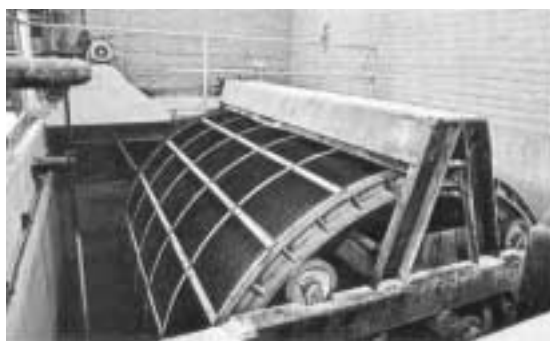
Figure 8-63(a) Microscreening process. (Courtesy of U.S. Filter/Envirex Products.)
