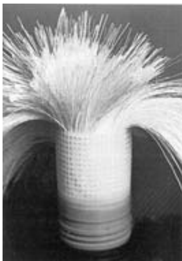
Figure 8-65(a) Commercial membrane configurations. (Courtesy of U.S. Filter/Memcore.)
