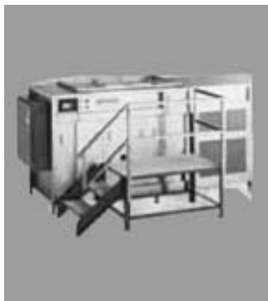
Figure 4-1 Photograph of a typical vapor degreaser. (Courtesy of Greco.)
