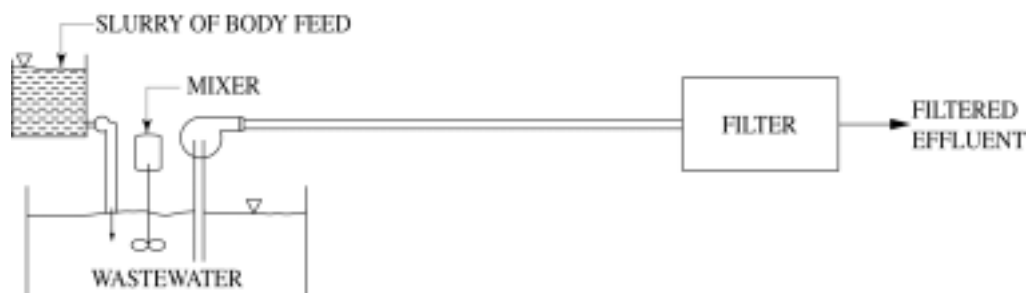
Figure 8-71(b) Body feed added in mixing tank.
