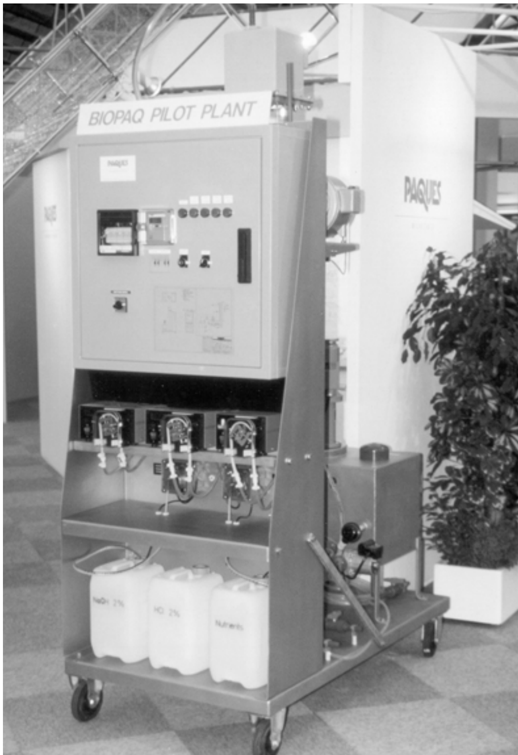
Figure 1-4 Photograph of a pilot scale wastewater treatment system. (Courtesy of Paques ADI, Inc.)
