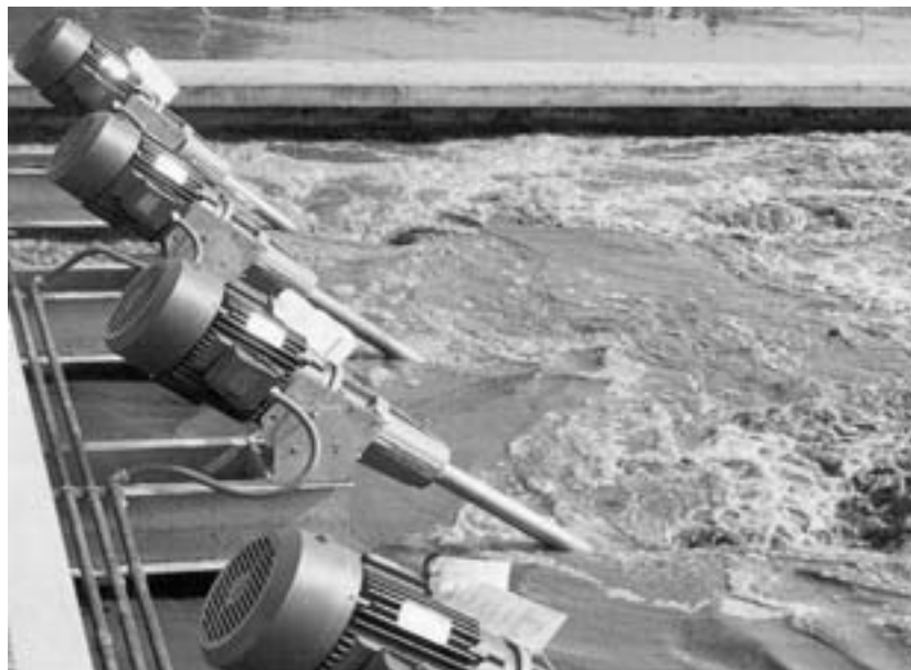
Figure 8-38(l) Alternative device for aeration: Fixed-mounted, aspirating aerators. (Photo courtesy of Eimco Process Equipment, a Baker Hughes Company.)
