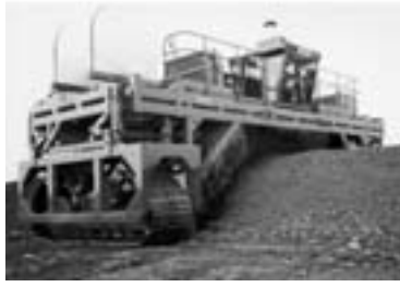
Figure 9-14 Windrow composting machine. (Courtesy of Scarab Manufacturing.)
