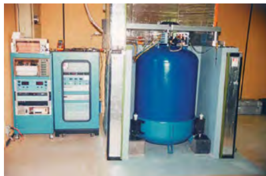
Figure 1 An example of the TT70 type instrument installed at Cantley, Canada, in 1989. The rack on the far left contains the chart recorders and noncritical electronics; the more sensitive components are in the enclosed temperature-controlled rack next to it. The 200 l dewar sits on three feet placed on small granite blocks. The front two feet with the X and Y thermal levelers attached to the dewar bottom are visible. The coldhead is supported from a frame resting on the top of a concrete pier. Normally, the entire SG is enclosed by thermal insulation.
