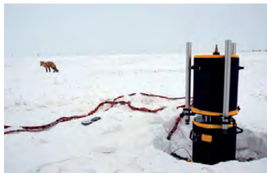
Figure 18 A10 deployed in Prudhoe Bay, from MicroLacoste.
